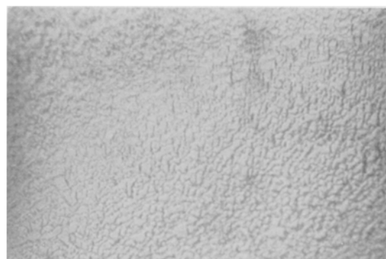
Fig. 6. Polycrystalline deposit on the copper (III) plane from the acid sulphate bath with 10^{-4} M 2-thiouracil at 10 \text{ mA cm}^{-2} . \times 600 .
