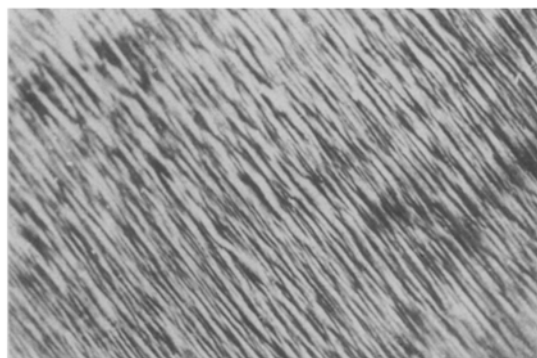
Fig. 5. Ridge type of growth on the copper (III) plane from the acid sulphate bath with 10^{-3} M 2-thiouracil at 10 \text{ mA cm}^{-2} . \times 600 .
